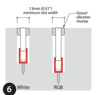
Finish slots between product and channel material with suitable filling product, such as grout, silicone or mortar.
