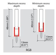
PVC channel accessory can be used to install GROOVE Light into a recessed channel at any orientation, 30mm (1.18") to 38mm (1.5") for white or 40mm (1.57") to 48mm (1.89") for RGB recess depth by 13mm (0.51") width.
