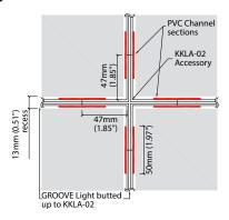
The above diagrams show the recommended clip/channel mounting positions for KKLA-01 and KKLA-02 in plan view. The width of the recess will be dictated by the clip used, in this example the PVC channel is used for mounting. Please refer to clip details above for recess depth and width requirements based on mounting method.
