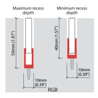
GROOVE Mini Clip accessory can be used to install GROOVE Light into a recessed channel at any orientation, 30mm (1.18") to 40mm (1.57") for white or 40mm (1.57") to 50mm (1.97") for RGB recess depth by 10mm (0.39") width.
